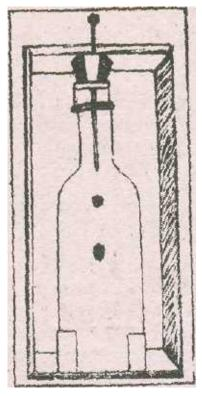
b) Model 2- The ends of the bottle are inserted into the holes made in two thick pieces of wood, and a thin piece of wood is fixed across the outside of each opening to prevent the article from passing through. The two pieces are then screwed to a base board which again is screwed to the base of a wooden box—see the figure given below.
